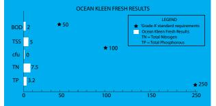
As shown by the graphs the quality of the effluent produced by the Ocean Kleen far exceeds the 'Grade A' Standard, with Ocean Kleen Fresh exceeding Advanced Secondary.
